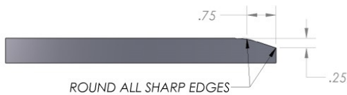
SPIGOT BEVEL DETAIL
